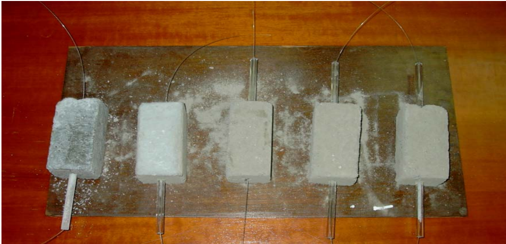
Figure 1: Samples of reinforced mortar prisms
